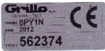
The rotavator is fitted with a nameplate on the frame with the serial number of the machine. Always state the serial number when ordering spare parts or asking for technical support.
