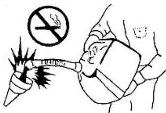
*Handle fuel with care, it is highly flammable: Do not refuel machine while smoking, when machine is near an open flame or sparks, or when engine is running. Stop engine.*
