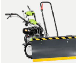
Pala frontal orientable, 100 cm GH 8 - GH 9
